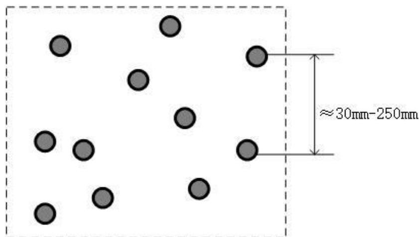
Figure4- 1 Pasting uncoded markers
