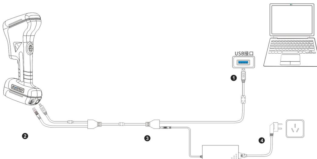
Figure2- 11 Device connection
